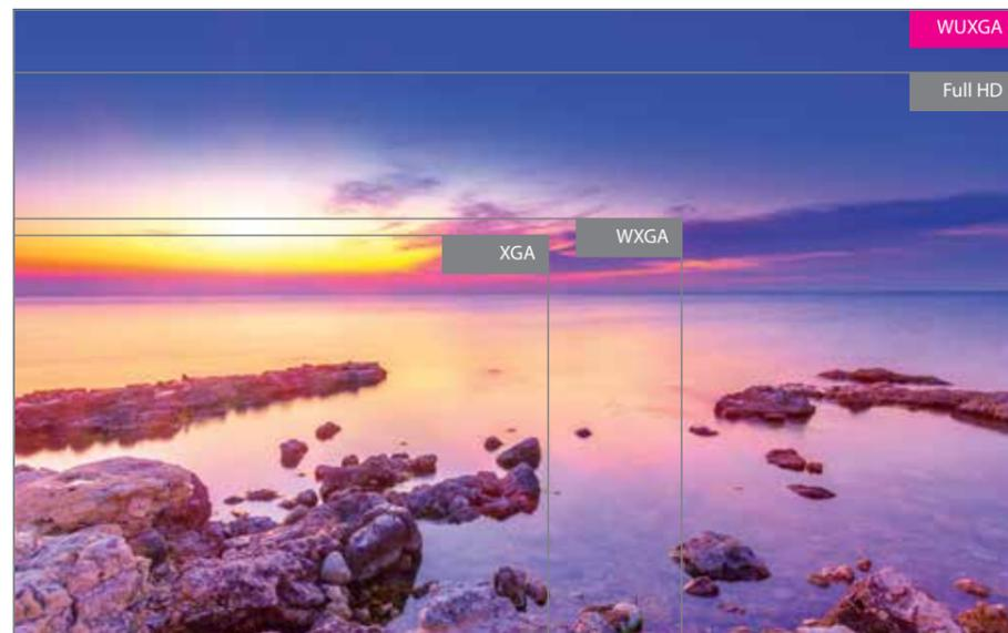
When detail really matters, WUXGA resolution (1920 x 1200 pixels) offers 15% more image area than 1080p and 60% more than SXGA+. This enables unscaled Full HD video and extra detail. Time code information can be displayed on-screen at the same time, perfect for soundtrack recording and video editing editing where precise timing can be critical.
