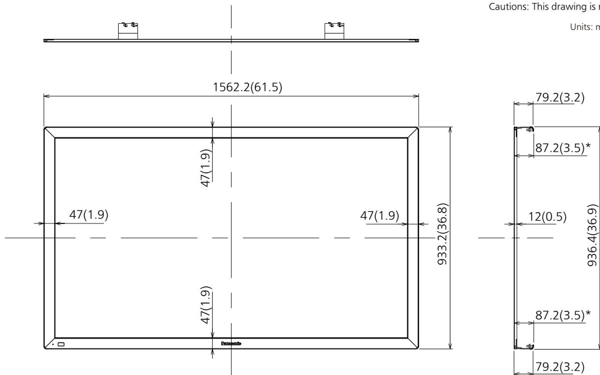
\*Dimensions may vary by the mounting set and the tightening state.
