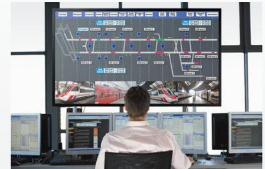
A 4K display panel can be set up in a room with limited space since the optimum viewing distance for 4K images is shorter than that for HD.
